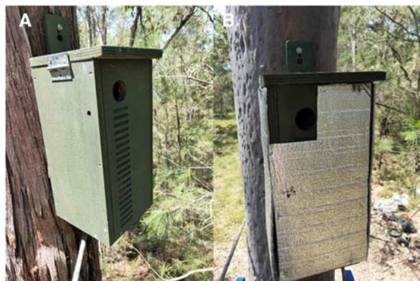
Figure 2: Photographs of nest boxes installed on trees without insulation (A) and with 4-mm reflective aluminium insulation (B).
